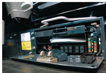
Fan belts are accessible through a hatch to the right of the cabin. The battery is protected by a metal plate behind the right back cover. The electrical components are under the seat.
