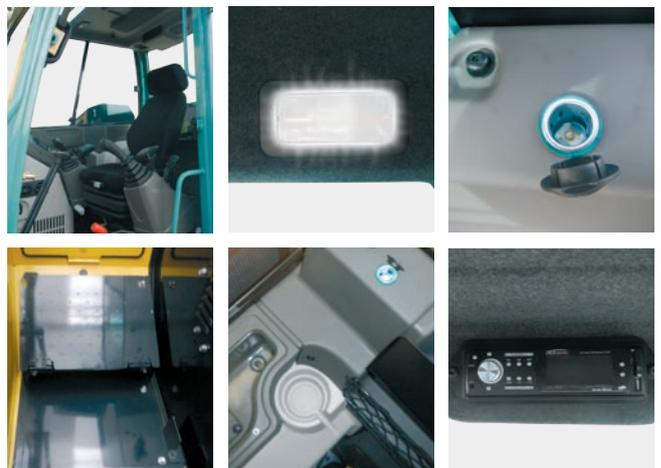
Standard equipment also includes: a radio with USB port, several handrails, numerous storage spaces, an automatic ceiling, a bottle holder, two 12-volt sockets, a coat rack, a toolkit...
